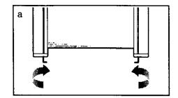
b. If the walking belt has shifted to the right, first remove the safety key and UNPLUG THE POWER CORD. Using the 3/16" allen wrench, turn the left rear roller adjustment bolt counterclockwise, and the right bolt clockwise, 1/4 of a turn each. Be careful not to overtighten the walking belt. Plug in the power cord, insert the safety key and run the treadmill for a few minutes. Repeat until the walking belt is centered.
